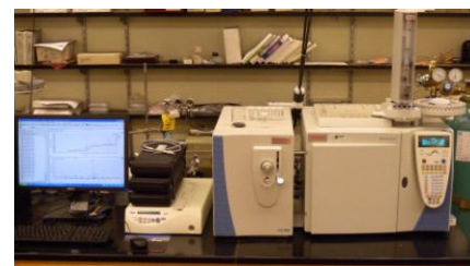
The new Thermo Finnigan iTQ-1100 GC-MS, which was installed last January, is housed in the Advanced Instrumentation Lab due be renovated.
