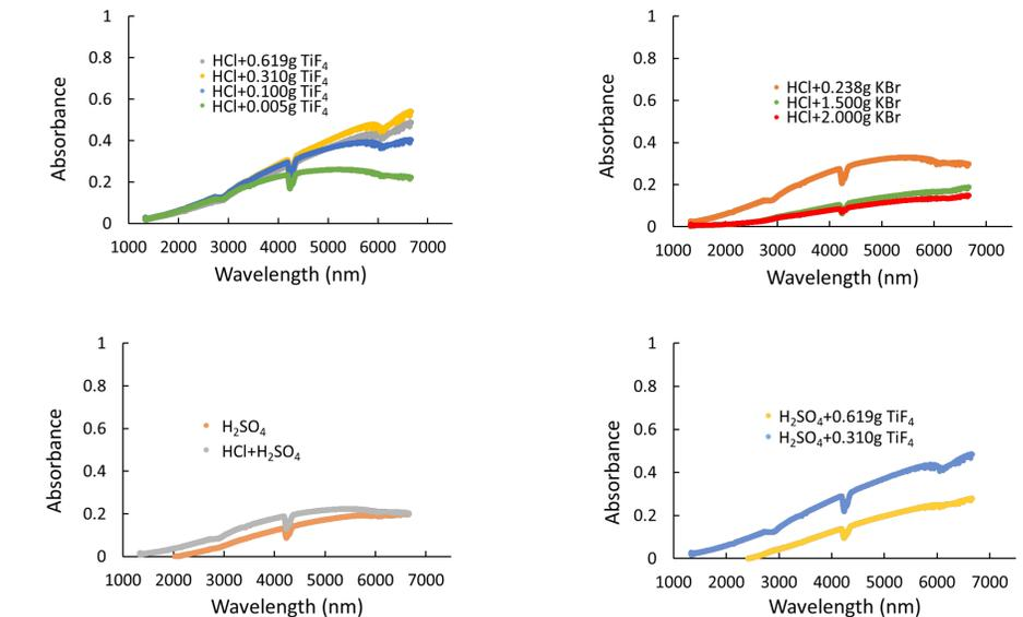
Anions could effectively control the crystallization process and the surface reconstruction, and therefore change the light absorption properties. Our UV-Vis study showed that F<sup>-</sup> could significantly increase the overall absorption while Br<sup>-</sup> could suppress the visible light absorption. Therefore, we mixed F<sup>-</sup> and Br<sup>-</sup> to fine tune the optical properties.
