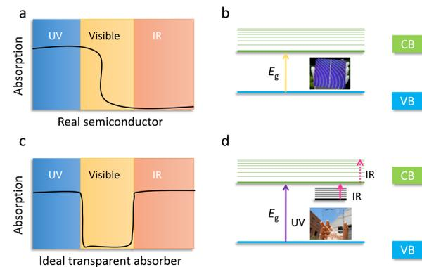
Figure 1 Scheme of band structure engineering for transparent absorbers.
