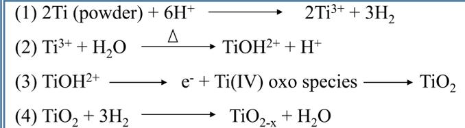
TiO<sub>2-x</sub> represents the final product where the 2-x indicates that the oxygen vacancy. Therefore, the TiO<sub>2-x</sub> is TiO<sub>2</sub> doped with Ti<sup>3+</sup>.
